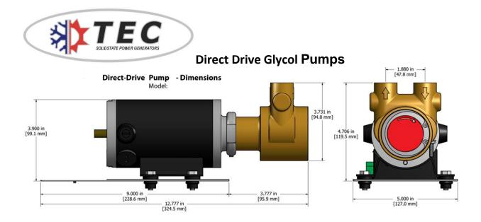
The Direct-Drive Glycol TEG Pump<sup>™</sup> (model: 330-2407112P) is a Glycol TEG Pump<sup>™</sup> and features a brushed DC motor, and a standard size pump head (model: TP330). Flow rates range from 2.0 liters/minute (0.5 USGPM) to 12 L/m (3.2 USGPM). Available in 12 & 24 VDC configuration.
