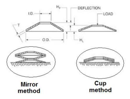
Belleville Washers are design for maintaining constant compression on TEG modules during thermal cycling. To install correctly, use 2 washers according to (cup method) illustrations above. Either a mirror method or cup method can be used, but it is recommended 2 washers be used per screw for proper deflection.
