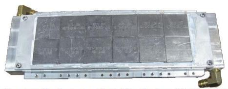
Liquid sinks with outstanding heat removal capability. Single and double sided sinks available. The sinks will hold 12 pieces 40mm x 40mm modules. The sinks are designed for liquid to contact all modules in parallel, thereby not compromising the DT to modules at the end of the flow channel. Whale fin® Patent Pending
