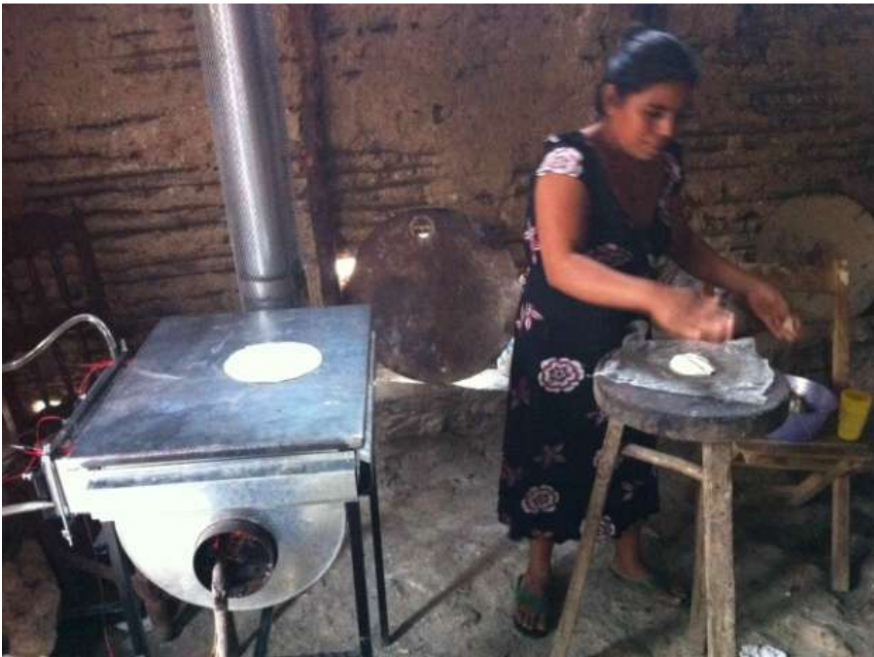
14 to 17 watt Liquid TEG located on the left side of the stove
