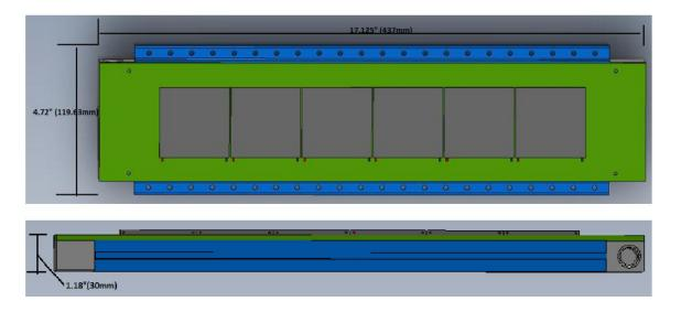
\*\* Because of our large flow surface under the modules of the cold interface plate. The correct number of modules are required for proper operation of the liquid sink. Failure to use 4 x 56mm modules in this case will reduce counter pressure on the O-ring which may cause it to leak.
