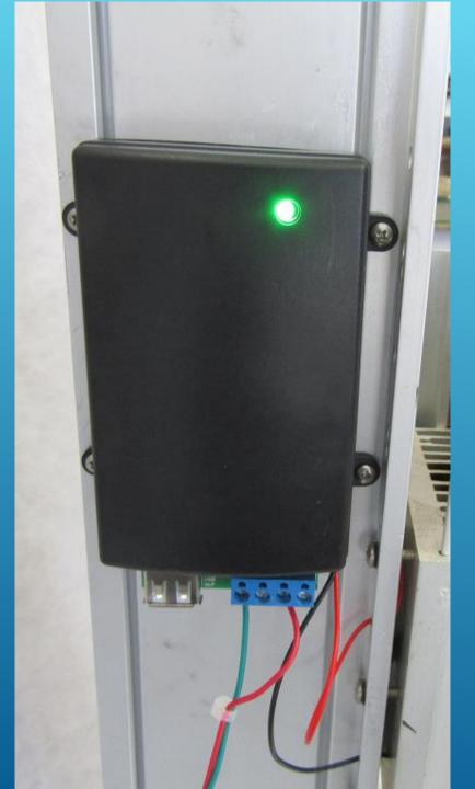
The green light will turn on when the system reaches charging power strength. Because of the large mass heat sink it takes about 3 to 4 minutes.
